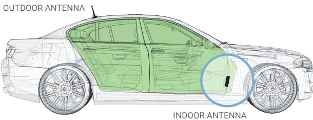
Install **Indoor Antenna** in the cab, towards the front, where coverage is needed. Ideally, there should be substantial material, like the metal of the roof, between the **Outdoor** and **Indoor Antennas**, to improve isolation.
