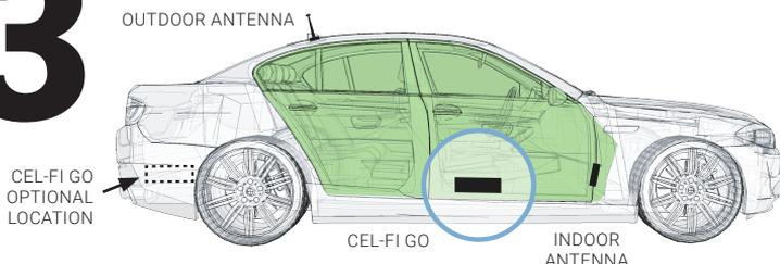
Find a good mounting location in your vehicle. Location should have some airflow, and be safe from bumps and external objects.
