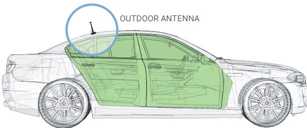
Mount your **Outdoor Antenna** on the exterior of the vehicle, towards the rear, according to its design, and the type of vehicle it's being used with. Make sure you consider the cable connection to the **CEL-FI GO** unit with your location choice.
